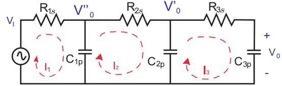
Figure 1: Low frequency Interconnect Model
