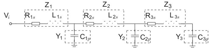
Figure 2: Interconnect model at high frequencies
