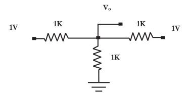
(b) For the same network determine Vo when the signal is differential.
