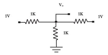
The concept of superposition theorem and splitting any signal pair into common mode and differential mode part is illustrated in the next example. The concept of common mode input resistance and differential mode input resistance can be explained and evaluation of common mode rejection ratio can be carried out.
